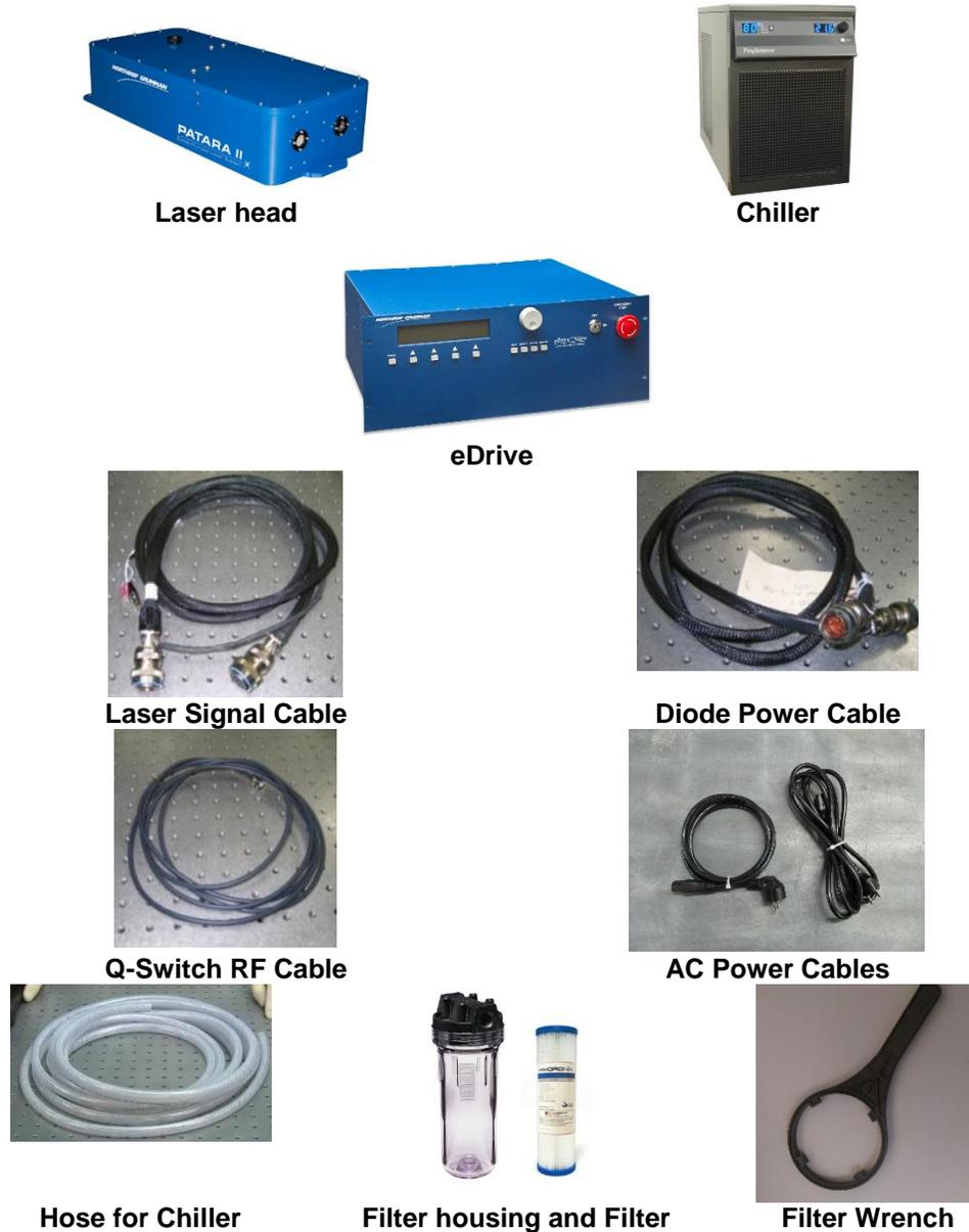
**Figure 4-1.** Components for the Patara Laser
