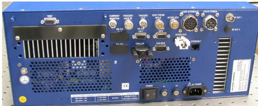
Figure 4-10. Rear Panel of the eDrive
